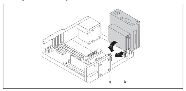
► Gently press the upright bracket (b) of the drive cage in the direction of the arrow (1) until you can move the drive cage.
